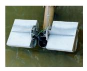
Procedure 2 The Hydro-Surf Decanter with integrated turbidity measurement drains away the clean water under the floating solids zone. Either through gravity or by means of a pump, it conducts the clean water
