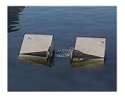
Procedure 1 The Hydro-Surf Skimmer draws the floating solids and light density matter from the water surface for treatment
