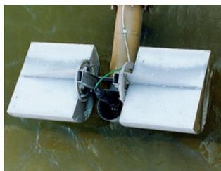
**Procedure 2** The **HydroSurf Decanter** with integrated turbidity measurement drains away the clean water under the floating solids zone. Either through gravity or by means of a pump, it conducts the clean water
