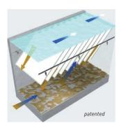
The HydroM.E.S.I.® Particle Separator is specially designed to deal with particle-based water pollution. Whilst in operation the lamellae plates are submerged; the pollutant impurities are bonded to the fine suspended solids. These solids are settled to
